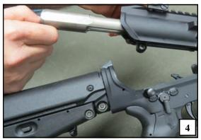
Remove the bolt carrier group simply by pulling it rearward from the upper group. Note: Unlike other AR10 style rifles, the charging handle will not interfere with removal and installation of the carrier group.
