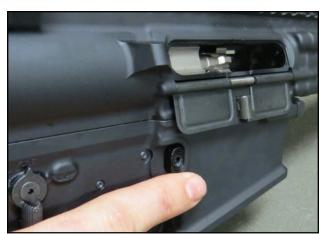
**Note:** You do not need to press the forward assist button to charge the rifle.
