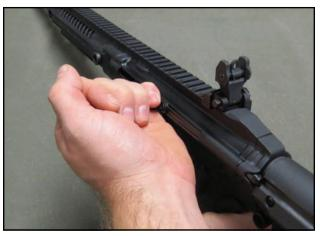
**Note:** You will not be able to engage the safety selector to the "SAFE" position if the rifle is not already charged, an it will remain in the "FIRE" position. If the rifle is already charged you should engage the safety selector to the "SAFE" position at this time.
