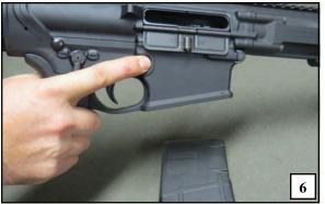
Once a firing session is complete, to drop the magazine press the magazine release button as shown in the picture above. The magazine will normally fall out under its own weight, so be careful that it does not become damaged or lost when falling.
