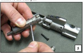
Use the firing pin to remove the extractor pin. At this time, inspect the firing pin for bending, damage or deformation to the spherical surface of the primer striking tip, and excessive mushrooming on the hammer strike face.
