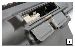
Clear your weapon. Pull the charging handle back and ensure the chamber is empty. Once verified empty, allow charging handle to slide bolt carrier group forward.
