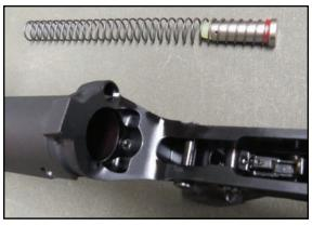
To reinstall the buffer assembly and recoil spring you do not need to push down the buffer retainer pin, as the spring and buffer body will automatically push it down.
