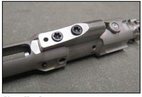
Piston Key Screws: Torque value: 55 in-lbs
