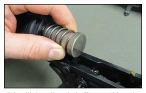
This will then allow the buffer assembly and recoil spring to be removed from the buffer tube. **Note:** Be careful that the buffer assembly does not spring out with enough force to damage or ding other components on the rifle.
