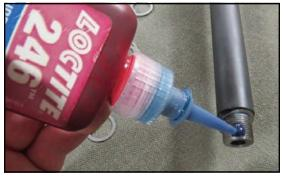
Once a shim value is determined, remove the device and apply 246 Loctite to the muzzle threads then reinstall the muzzle device and tighten until the desired alignment is attained.
