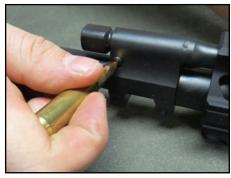
This section reviews the adjustment procedure for F&D's proprietary patent-pending gas system. To open the gas valve retaining pin, use a crimped bullet to slide the pin over to the open position. This will allow rotation of the gas valve to any desired primary settings and will allow removal of the gas valve and other gas system components. The setting that is positioned upward is the setting applied to the gas system.
