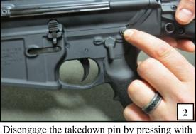
Disengage the takedown pin by pressing with your finger or a crimped bullet and sliding to its fully open position.
