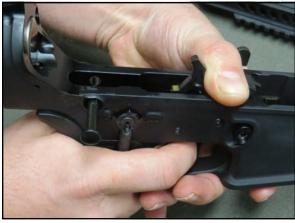
If the trigger feels "notchy" as it comes to the second stage there is not enough sear engagement, therefore you must turn the sear adjustment screw another 5-10 degrees clockwise or until the notchy feeling is eliminated.
