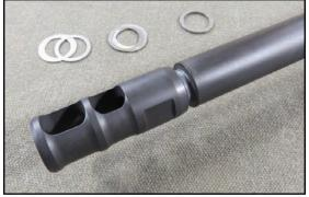
Thread the muzzle device onto the barrel without any shims and tighten as you would for general operation. This will provide an indication of the required amount of angle the shims need to reverse-clock the muzzle device.
