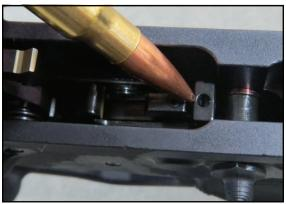
Once no second stage exists, rotate the sear adjustment screw clockwise while repeatedly cocking the hammer and pulling the trigger. Only 10 degree turns are required during this process.
