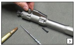
Remove the cam pin.
