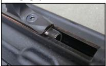
FD platform rifles incorporate a unique charging system built around a sliding rod instead of a sliding rail system. This allows the mechanical system to operate smoother, more reliably, and easier to maintain than all other charging systems. The handle has a consumable bronze
