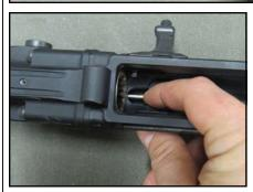
Slide the piston rod (or direct impingement gas tube) towards the muzzle end of the rifle. The piston will then be pushed out of the gas block, ensure you catch the piston as it comes out to avoid losing or damaging it.
