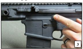
To charge the rifle and load a round into the chamber, press the bolt catch button. Ensure the rifle is pointed in a safe direction and away from objects that could otherwise cause bullet ricochet into an unsafe area.
