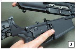
The upper group will be allowed to pivot. Note: Unlike other AR10 style rifles, there is no concern with damaging the port cover on F&D rifles during pivoting, so the port cover can remain open.
