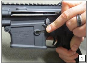
Without a magazine installed, pre-charge the rifle and engage the bolt catch as shown.
