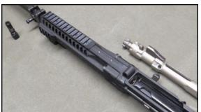
Remove the upper group from the lower group, then remove the bolt carrier assembly. This will provide access to the piston rod (or direct impingement gas tube) from inside the upper receiver.
