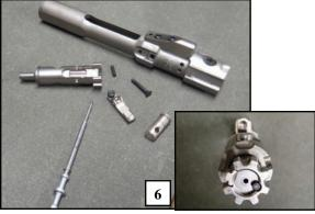
Reassemble the bolt carrier group in the reverse order it was assembled. **Note:** shim washers may be installed on the firing pin, as shown in the above picture, which will allow the ability to attain a desired depth in which the firing pin engages the primer.
