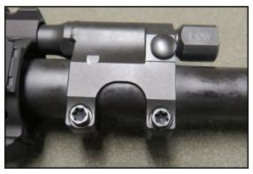
Gas Block Screws: Torque value: 55 in-lbs
