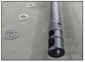
Once an angle is established, divide it by 360 and multiply by thread pitch (.0417).
