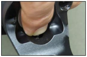
To remove the buffer assembly, press the buffer retainer pin down with your fingernail or a crimped bullet tip.
