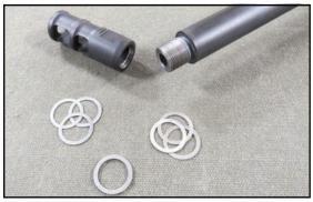
Shims are required in order to attain a desired clocking angle for brake-style muzzle devices. Contact F&D for a shim kit if necessary, which will allow clocking for and device on any F&D rifle. The kit consists of one .046", three .005", and three .006" shims.
