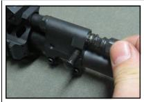
As described in the gas valve settings section on page 17, disengage the gas valve retaining pin by sliding to its fully open position. Now the gas valve is free to be rotated or removed from the gas block. If, after extended periods of sustained fire the gas valve becomes seized, apply a carbon-binding penetrating oil and allow to soak for
