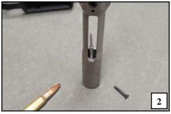
Once the retainer pin is removed, the firing pin will drop from the assembly. Tap the assembly in the orientation shown above if the firing pin does not freely fall from the bolt carrier group.
