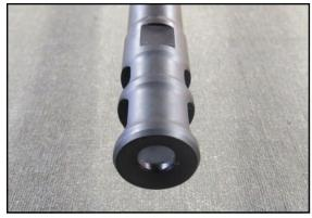
The muzzle device should now be clocked horizontally as shown above within approximately 5-10 degrees.
