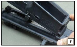
To remove the lower group from the upper group, disengage the pivot pin by pressing with your finger or a crimped bullet and sliding to its fully open position. The lower group will then be completely disconnected from the upper group.
