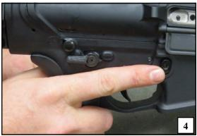
The rifle is now charged with a live round in the chamber. Until you are ready to engage targets, the safety selector should be set to the "SAFE" position and your finger should be off the trigger and out of the trigger guard area.
