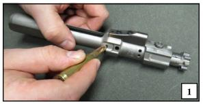
Use a crimped bullet tip to remove the firing pin retainer. Using a razor blade you may adjust the fit of the retainer pin by flaring the slot.
