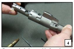
Remove the bolt assembly from the carrier.
