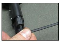
The gas-valve regulating needle is adjusted with a 5/32" allen wrench (preferably an extended ball driver style). First, remove the setscrew that locks the regulating needle in place. **Note:** Check the tightness of
