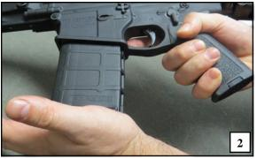
Load a magazine. Note: F&D rifles are designed with a snug fit on Magpul magazines, and you may need to snap the bottom with the palm of your hand in order to fully engage.
